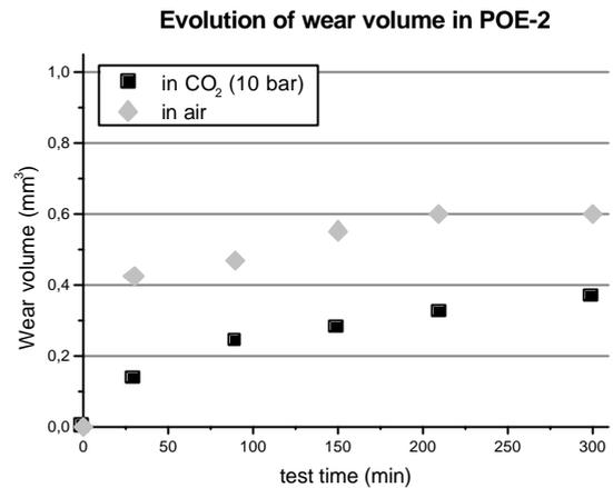
Figure 9 : Evolution of wear volume of POE-2 in air and in compressed CO<sub>2</sub>
