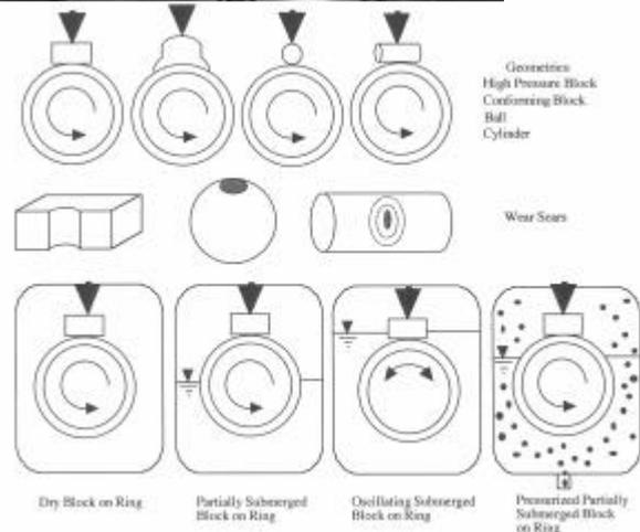
Figure 2: Block-on-ring test machine with pressure chamber. Contact geometry (above) – possible configurations (below)
