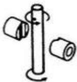
Figure 1 : Schematic of the Pin&Vee Block test method
