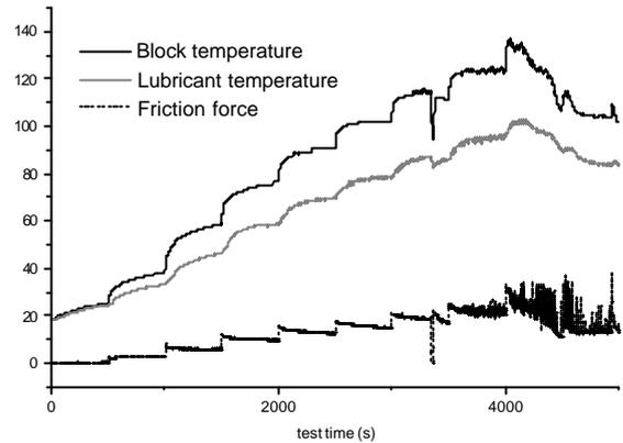
Figure 6 : Online data during Block-on-ring EP test in air, POE-0, steel block vs. steel ring
