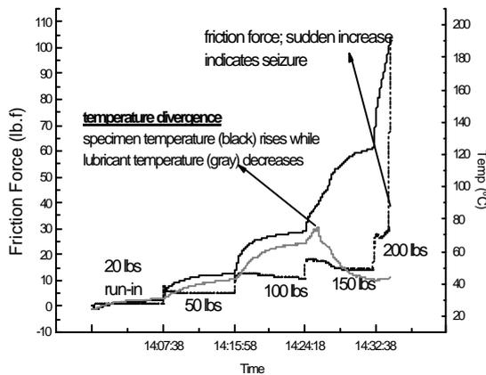
Figure 3 : On-line friction force in the extreme pressure Block-on-ring test, steel block. Immediate increase in friction force when lubricant film breaks down.
