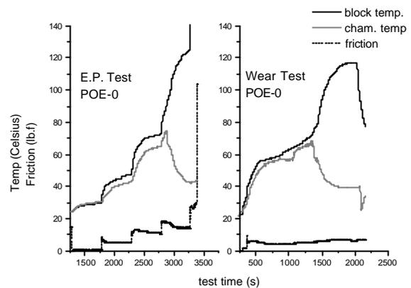
Figure 7 : Online data during Block-on-ring EP test (left) and Wear test (right) of POE in 10 bar CO<sub>2</sub>.
