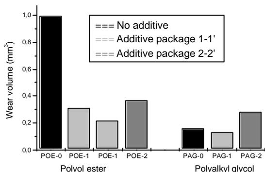
Figure 11 : Wear volume after 5 hour tests in CO<sub>2</sub> for different synthetic lubricants and additive packages.
