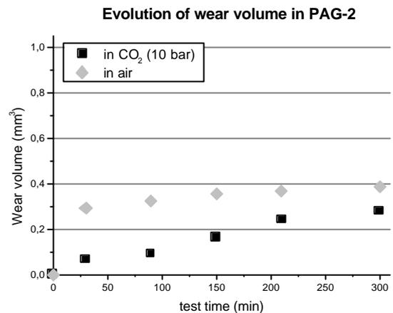
Figure 10 : Evolution of wear volume of PAG-2 in air and in compressed CO<sub>2</sub>
