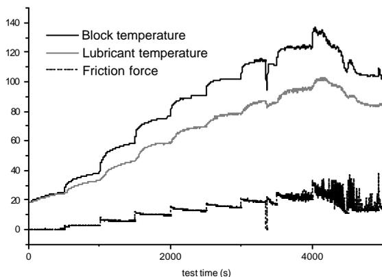
Figure 6. Every time the load on the contact is increased, the frictional force increases also leading to higher frictional heating. As the temperature of the
