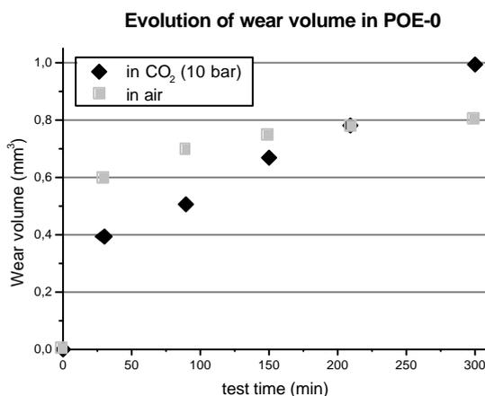
Figure 8 : Evolution of wear volume of POE-0 in air and in compressed CO<sub>2</sub>
