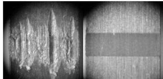
Figure 5 : Left : seizure of Aluminium test block in Block-on-ring E.P. test. Right : uniform wear of Steel test block.
