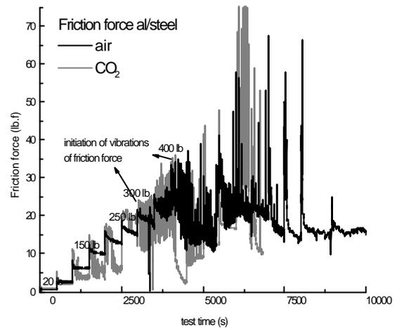
Figure 4 : On-line friction force in the extreme pressure Block-on-ring test, steel block. Breakdown of lubricant is indicated by incipient seizure (friction signal showing large variations)
